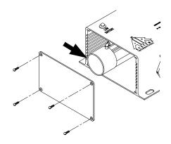
**STEP 1)** Disconnect all external connections. Remove CO monitor from the unit.
